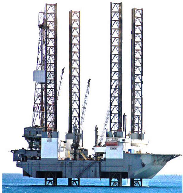
Figure 16: Jack-up Drilling Rig
