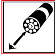
4. Use the appropriate comparator to determine the level of copper in the sample. If the color of the CHEMet ampoule is between two color standards, a concentration estimate can be made.
