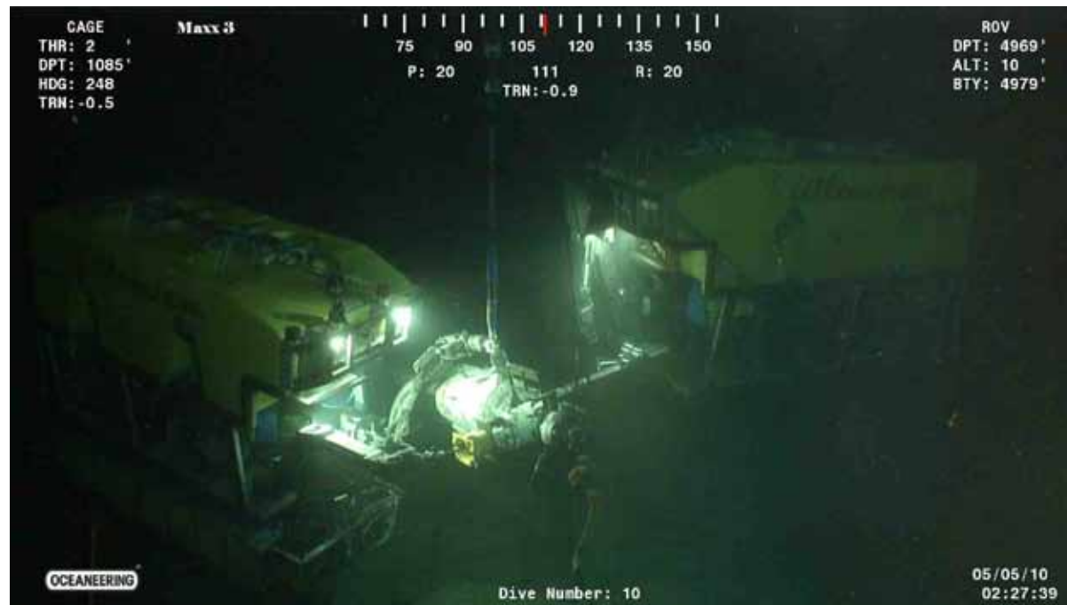
Remotely Operated Vehicles (ROVs) closing the valve on the end of the damaged riser pipe. Advancements in ROV tooling and subsea hydraulic distribution permitted highly efficient ROV operations.
