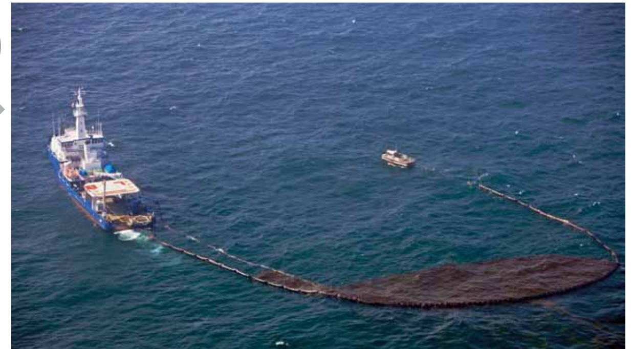
At the peak of the response more than 60 open-water skimmers were deployed within an innovative “command and control” system which combined air intel with on-water, central coordination of skimming traffic for optimal vessel placement.
