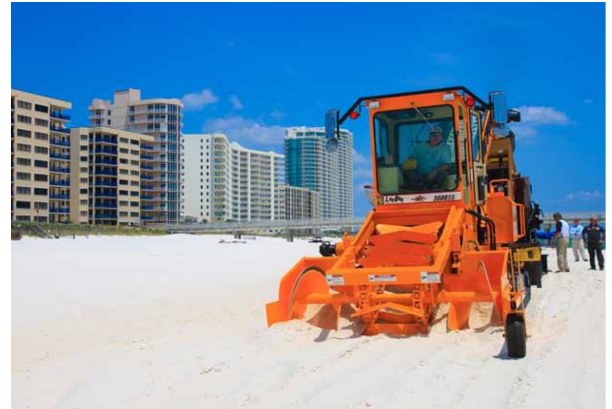
A Sand Shark developed specifically for the beach clean-up effort, using continuous improvement methodology, allowed deeper digging to capture oil below the surface.
