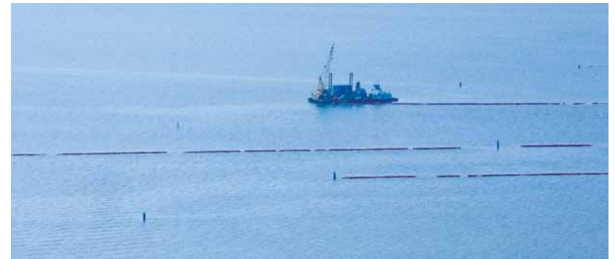
A vessel deploys boom. The response team cooperated with government officials and environmental experts to maximize the use of boom while ensuring appropriate placement and application.
