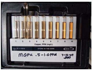
Copper PPM Level is Between 2-3 PPM Need to adjust Amperage Setting so that PPM Level is between .5 and 1 PPM
