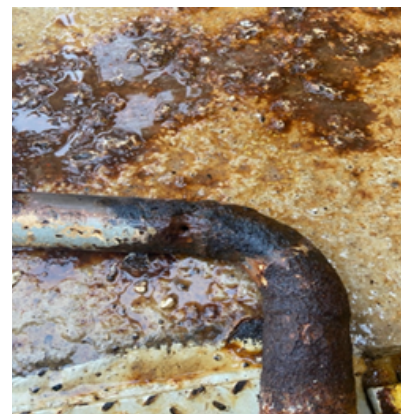
Identification of leak located under deck and encased in thermal insulation that could not be seen. Pipe condition after removing thermal insulation
