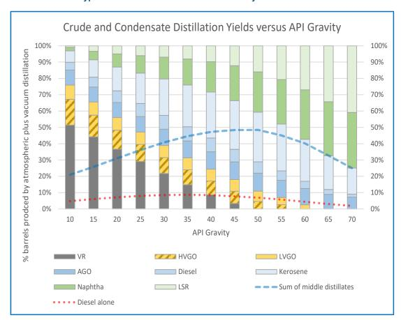
Exhibit 4: Typical Distillation Yields versus API Gravity of Crude and Condensates
